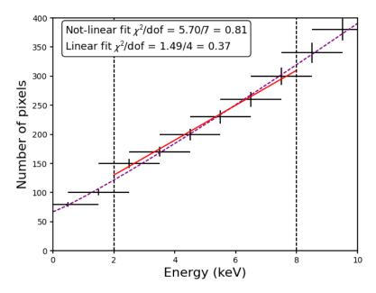
**Figure 6.** Threshold on the number of pixels — for which the source events above it are negligible — as a function of energy (black points). The purple dashed line shows a best-fit in the 0–10 keV energy band for the function 4, and the red line is a simplified linear function valid in the 2–8 keV IXPE nominal energy band.
