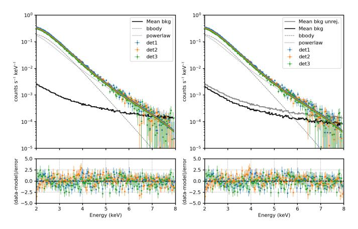
**Figure 19.** 4U 0142+61 data fitted with XSPEC before (left) and after (right) the background rejection; the considered spectral model is TBABS\*(BBODY+POWERLAW). At the bottom, residuals with respect to the best-fit model are shown. On the right panel, the background before and after rejection are compared, and it is possible to appreciate its reduction after the rejection procedure.
