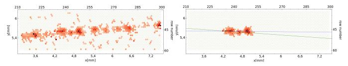
Figure 7. Example of a track with more clusters (left), where only the one reported in the right panel is considered for the track reconstruction by the IXPE algorithm.
