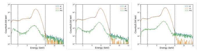
**Figure 14.** Energy spectrum from Cal C in the three detectors of IXPE, from left to right: DU1, DU2, DU3. In each plot, the spectrum without rejection (blue line) with label all is compared with the one of events tagged as source (src) after rejection (orange line) and the rejected events tagged background (bkg, green line).
