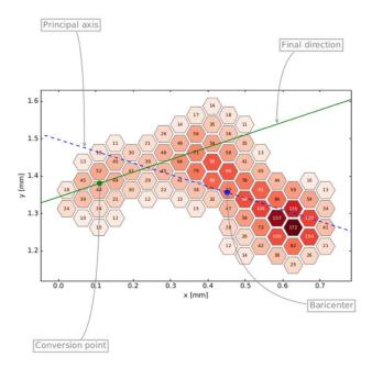
Figure 1. An example of an ionization track resulting from absorption of a 5.89 keV X-ray, as amplified by the GEM and imaged onto the GPD's pixelated anode — a  $300 \times 352$  array of hexagonal pixels at 50  $\mu$ m pitch (Sgrò 2017).
