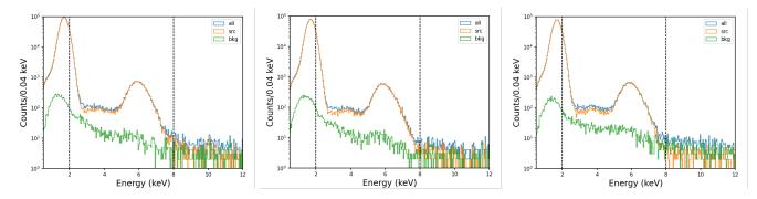
**Figure 15.** Energy spectrum from Cal D in the three detectors of IXPE, from left to right: DU1, DU2 and DU3. In each plot, the spectrum without rejection (blue line) with label all is compared with the one of events tagged as source (src) after rejection (orange line) and the rejected events tagged background (bkg, green line).
