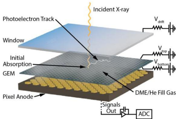
Fig. 2. Schematic of the polarization-sensitive gas pixel detector.
